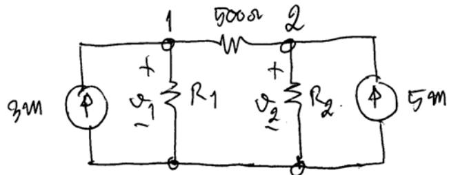
$$\text{At Node } \#1; \frac{v_1 - v_2}{R_1} = 0.003 \quad -\textcircled{1}$$
